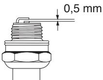
**CAUTION!** Always use the recommended spark plug type! Use of the wrong spark plug can damage the piston/cylinder.
