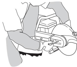
Tightening torque for the bolt holding the blade is: 15-25 Nm (130-215 in.lb).
