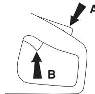
The trigger lock remains pressed in as long as the throttle is pressed. When the grip on the handle is released the throttle trigger and the throttle trigger lock both return to their original positions. This is controlled by two independent return spring systems. This means that the throttle trigger is automatically locked in the idle position.
