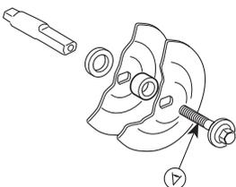
Do not use warped, notched, indented or dirty flange washers. Do not use different dimensions of flange washers.
