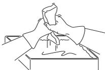
Put the filter in a plastic bag and pour the filter oil over it. Knead the plastic bag to distribute the oil. Squeeze the excess oil out of the filter inside the plastic bag and pour off the excess before fitting the filter to the machine. Never use common engine oil. This would drain through the filter quite quickly and collect in the bottom.
