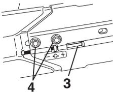
Screw in the tension screw (3) so that the square nut aligns with the arrow on the belt guard. Shake the head to ensure the spring can tension the belt. This automatically adjusts the belt to the correct tension. Tighten both bolts (4) using the combination spanner. **NOTE!** When a belt is fitted the belt tension must be readjusted after the first two tanks of fuel have been used.
