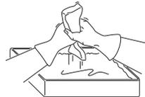
After cleaning the foam plastic filter needs to be oiled. See instructions under the heading Oiling the foam plastic filter.
