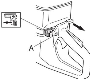
**Decompression valve:** Press in the valve to reduce the pressure in the cylinder, this is to assist starting the power cutter. The decompression valve should always be used when starting. The valve automatically returns to its initial position when the machine starts.
