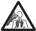
**WARNING!** Dust forms when grinding which can cause injuries if inhaled. Use an approved breathing mask. Always provide for good ventilation.
