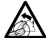
**WARNING!** Sparks from the cutting blade can cause fire in combustible materials such as: petrol (gas), wood, dry grass etc.
