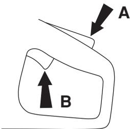
The trigger lock remains pressed in as long as the throttle is pressed.
