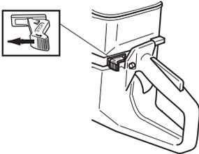
**Start throttle position - cold engine:** Start throttle position and choke is obtained by pulling out the choke completely.
