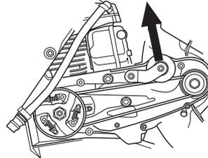
**CAUTION!** Make sure that both belt pulleys are clean and undamaged before a new drive belt is fitted.
