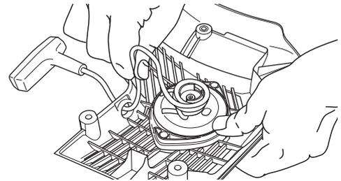
Now pull the starter handle and in doing so tension the spring. Repeat the procedure once more, but this time with four turns.
