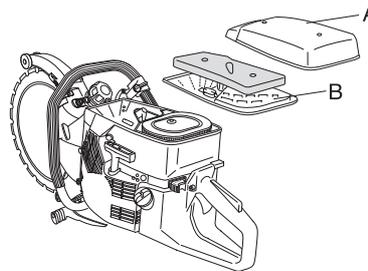
In order to obtain a good filtering effect, the filter must be replaced regularly or cleaned and oiled. A special HUSQVARNA oil has been produced for this purpose.
