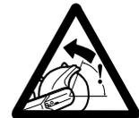
**WARNING!** Sparks from the cutting blade can cause fire in combustible materials such as: petrol (gas), wood, dry grass etc.
