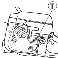
**Rec. idle speed:** 2500 rpm
