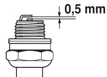
**CAUTION!** Always use the recommended spark plug type! Use of the wrong spark plug can damage the piston/cylinder.
