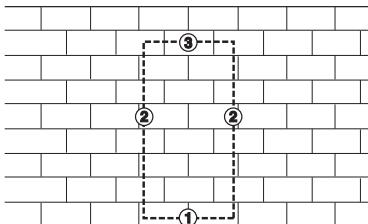
**CAUTION!** If the upper horizontal cut is made before the lower horizontal cut, the work piece will fall on the blade and jam it.
