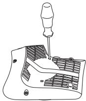
Bear in mind that the return spring lies tensioned in the starter housing. If the spring flies out during assembly, it is wound working from the outside towards the centre.
