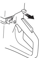
**Start throttle position - warm engine:** The correct choke/start throttle setting is obtained by pulling the choke control to the choke position and then pushing it in again. This only engages the start throttle setting without any choke.
