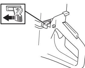
**Start throttle position - cold engine:** Start throttle position and choke is obtained by pulling out the choke completely.
