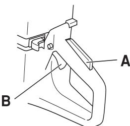
The trigger lock remains pressed in as long as the throttle is pressed.
