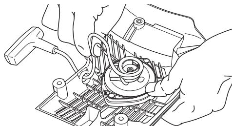
Now pull the starter handle and in doing so tension the spring. Repeat the procedure once more, but this time with four turns.
