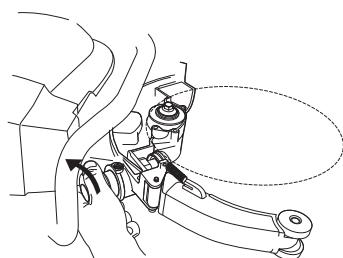
The guide roller can now be pulled out of the chassis
