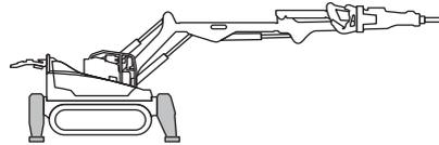
The main function of the outriggers is to give the machine stability. They must always be used when working with the machine.
