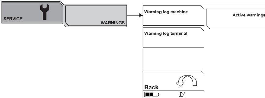
The machine has 2 warning logs and a list of active warnings.
