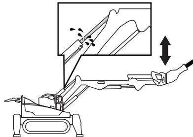
Cylinder 3 is in its outer position and the hammer is working in the downward direction. Never operate the cylinders to their end positions.
