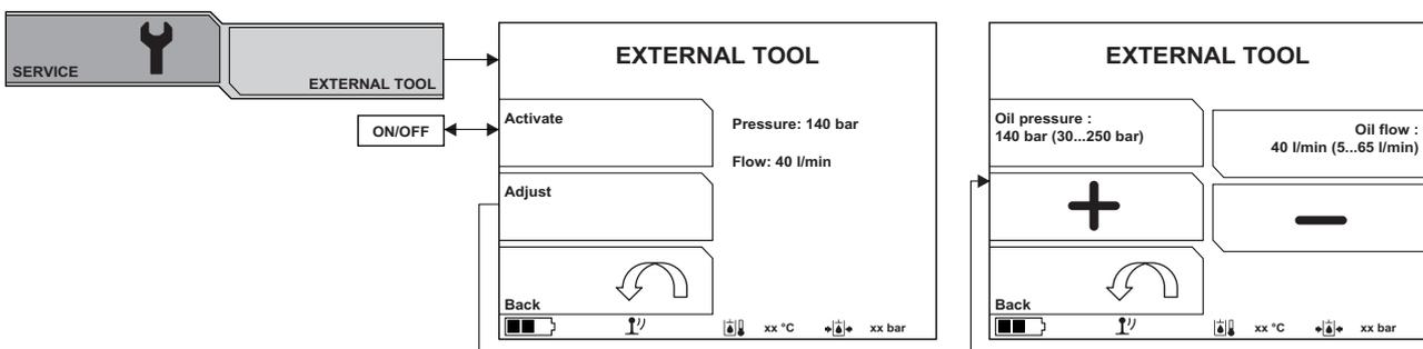
The machine can be used as a power source to operate external hydraulic tools.
