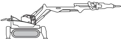
The caterpillar tracks are driven individually by hydraulic motors. The machine can be turned by operating the caterpillar tracks at different speeds. Operating the tracks in different directions enables the machine to make tight manoeuvres. When the drive function is not activated the passive brakes lock the drive motors.
