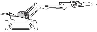
The tower can be turned indefinitely which makes it possible to work in several directions without having to move the machine.
