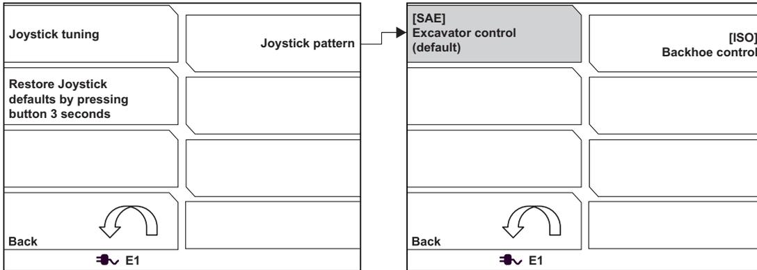
The joystick pattern changes the operation of the remote control. The operational pattern changes as below when the [ISO] Backhoe control is selected.
