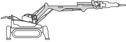
The arm system is divided into three parts in order to provide extensive movement, a long reach and compactness. Expanding shafts minimize the risk of play in the joints.
