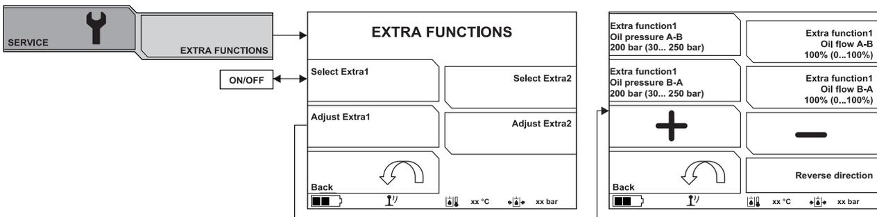
The machine can be equipped with extra valves to make it capable of running more functions, such as a rotor and a tilt.
