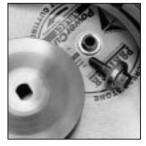
also prevents undesirable self-tightening. As usual, the lock-screw is right-threaded and features a permanent washer.
