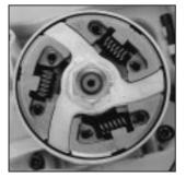
can no longer hold the shoes in place, and the shoes are pushed against the clutch drum by centrifugal force. Engagement speed is about 3400 rpm. At normal operating speed, centrifugal force is so high that a sudden overload on the cutter disc will cause the belt to slip against the pulley.
