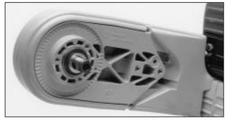
sealed casing that prevents water from reaching the belt. Dust is also kept away from the belt, thus reducing wear. In order for the transmission to be sufficiently cooled, the casing features cooling-air vents at the clutch.
