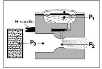
crease air resistance and promote a drop at  $(P_3)$  which is added to the pressure drop in the venturi  $(P_2)$ , so that the pressure differential compared with the carburettor's fuel chamber  $(P_1)$  increases. As a result, the carburettor enriches the mixture, supplying more fuel in relation to air, which in turn impairs the engine's performance.
