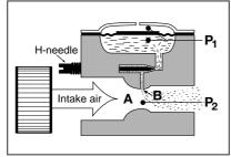
The carburettor's main job is to supply the right mixture of fuel and air to the engine. Every carburettor has a Venturi tube (A), in which the high speed jet (B) for petrol supply is fitted. When the engine sucks in air through the carburettor, the fuel is sucked down into the Venturi tube and mixed with the air.
