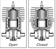
The cylinder bore is hard-chromed. The piston has two piston rings, and it has needle bearings at the coupling with the connecting rod.
