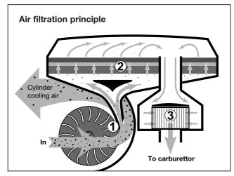
**1. Centrifugal force** is the first stage in cleaning the intake air of the K950/K1250 Active. Centrifugal cleaning was previously only used on larger engines in dusty environments, for example for construction machines (cyclone air filter).
