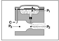
(P2) determines the amount of fuel which is to be mixed with the intake air. Therefore, irrespective of whether the filter system is clean or dirty, the relationship between air and fuel will remain constant at all times.
