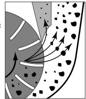
stead thrown against the outside of the nozzle. Only very small dust particles will be able to follow the current of air leading into the intake. Tests show that up to 80% of all dust is removed by the centrifugal cleaning process.
