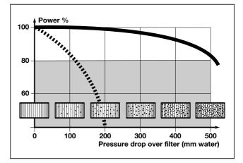
The above diagram (showing a laboratory test) demonstrates the considerable effect of SmartCarb<sup>™</sup> on engine power. Air pressure is measured at the carburettor's inlet and the figure 0 is set for brand-new filters and with the engine running at normal speed. As the filters accumulate dirt, the pressure drops owing to the increased build-up of air resistance.
