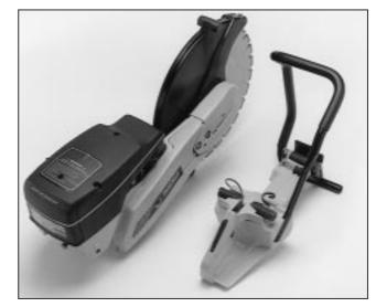
The four damper elements consist of steel springs with a rubber damper pad at the handle arch. The dampers are placed as far from each other as possible, thus achieving a good compromise between vibration suppression and operating convenience.
