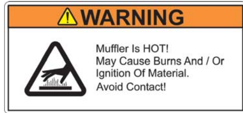
P/N 542 16 90-65 Location: Engine Fuel Tank, Near Muffler
