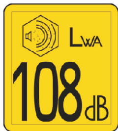
P/N 543 04 57-88 SOUND LEVEL - 108dBA Location: Blade Guard
