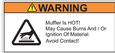
P/N 542 16 90-65 Location: Engine Fuel Tank, Near Muffler
