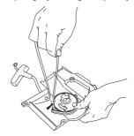
• Remove any remnants of the old starter cord and check that the return spring works. Insert the new starter cord through the hole in the starter housing and in the cord pulley.
