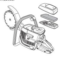
If the machine is low on power, difficult to start or runs poorly at idle speed: always check the spark plug first before taking any further action. If the spark plug is dirty, clean it and check that the electrode gap is 0.5 mm. The spark plug should be replaced after about a month in operation or earlier if necessary.
