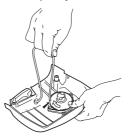
CAUTION! Check that the pulley can be turned at least a further 1/2 turn when the starter cord is pulled all the way out
