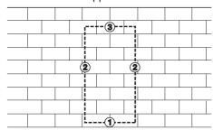
CAUTION! If the upper horizontal cut is made before the lower horizontal cut, the work piece will fall on the blades jamming them.
