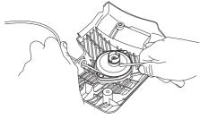
Secure the starter cord around the cord pulley as illustrated. Tighten the fastening well and ensure that the free end is as short as possible. Secure the end of the starter cord in the starter handle.
