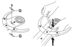
Refit the blades and tighten the nut. See instructions under Heading "Assembling the blades".
