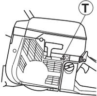
Rec. idle speed 2500 rpm
