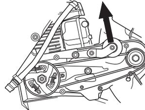
**CAUTION!** Make sure that both belt pulleys are clean and undamaged before a new drive belt is fitted.
