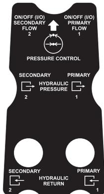
**DECAL, VALVE ON / OFF LOCATION:** VERTICAL SURFACE BELOW CONTROL PANEL
