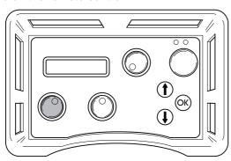
3. Start the horizontal motion by turning the horizontal motion knob in the desired direction.
