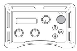
5. Set the feeding flow on the unit to max by turning the control on the remote control clockwise.
