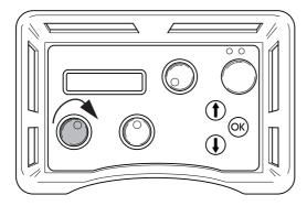
Tension the wire by carefully turning the knob on the pressure reduction block clockwise until the wire is tensioned sufficiently. Make sure to always check that the wire is seated correctly in all the wheels on the saw.
