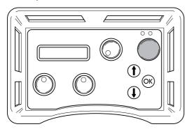
1. Turn the control for blade rotation to its maximum position to start blade rotation and the water coolant.
