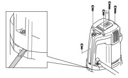
2 Lift the carbon brush holder spring to one side (A).
