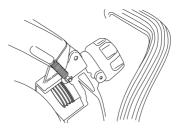
· Insert the guide roller in the chassis
