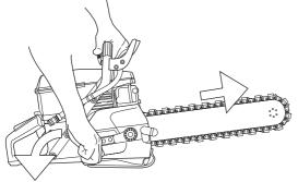
Hold the bar upwards as you move the handle forward.
