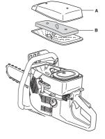
Remove the foam plastic filter. Wash the filter well in tepid soapy water. After cleaning, rinse the filter well in clean water. Squeeze out and allow the filter to dry. NOTE! High pressure compressed air can damage the foam.
