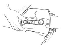
Press the spring down on the chain tensioner handle. Unscrew the adjusting bar nut anti-clockwise.
