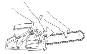
Lock the chain tension by tightening the counter screw.
