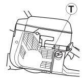
Rec. idle speed: 2700 rpm
