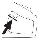
Press the throttle lockout and make sure it returns to its original position when you release it.
