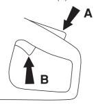
The trigger lock remains pressed in as long as the throttle is pressed. When the grip on the handle is released the throttle trigger and the throttle trigger lock both return to their original positions. This is controlled by two independent return spring systems. This means that the throttle trigger is automatically locked in the idle position.
