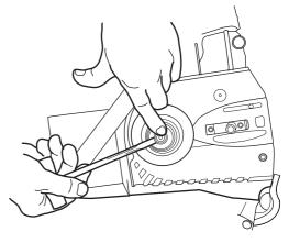
Remove the "halfmoons", the cup guard, o-ring and the drive sprocket.
