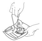
CAUTION! Check that the pulley can be turned at least a further 1/2 turn when the starter cord is pulled all the way out.
