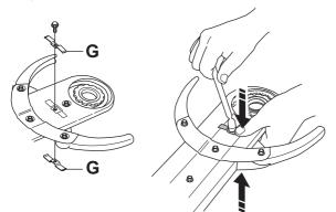
• Refit the blades and tighten the nut. See instructions under Heading "Assembling the blades".
