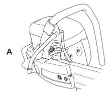
**Start throttle lock:** Press in the throttle trigger lock, throttle control and then the start throttle lock (B). Release the throttle control and it is locked in the half throttle position. The lock releases when the throttle control is pressed in fully.
