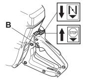
**Ignition:** Set the stop switch to the start position. **Choke:** Pull the choke control fully out.
