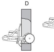
The blade guards are designed to easily adapt to how deep in the work piece the power cutter is moved.
