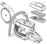
If the machine is low on power, difficult to start or runs poorly at idle speed: always check the spark plug first before taking any further action. If the spark plug is dirty, clean it and check that the electrode gap is 0.5 mm. The spark plug should be replaced after about a month in operation or earlier if necessary.
