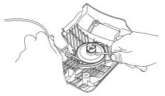
• Secure the starter cord around the cord pulley as illustrated. Tighten the fastening well and ensure that the free end is as short as possible. Secure the end of the starter cord in the starter handle.
