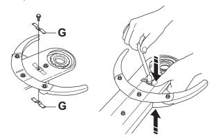
Refit the blades and tighten the nut. See instructions under Heading "Assembling the blades". CAUTION! Make sure that the belt adjuster screw bottoms and that the bar is fully screwed back so that the belt cover fits correctly.
