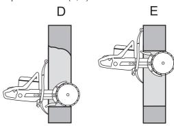
The blade guards are designed to easily adapt to how deep in the work piece the power cutter is moved.
