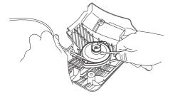
Secure the starter cord around the cord pulley as illustrated. Tighten the fastening well and ensure that the free end is as short as possible. Secure the end of the starter cord in the starter handle.
