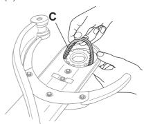
Loosen water hose (E). Slide back the bar and remove the drive belt around the clutch (D).
