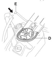
Pull off the cutting arm by pulling it straight forwards, as illustrated.
