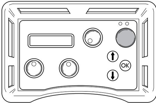
1. Turn the control for blade rotation to its maximum position to start blade rotation and the water coolant.
