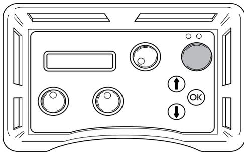
5. Set the feeding flow on the unit to max by turning the control on the remote control clockwise.
