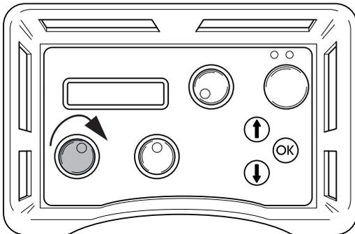
6. Tension the wire by carefully turning the knob on the pressure reduction block clockwise until the wire is tensioned sufficiently. Make sure to always check that the wire is seated correctly in all the wheels on the saw.
