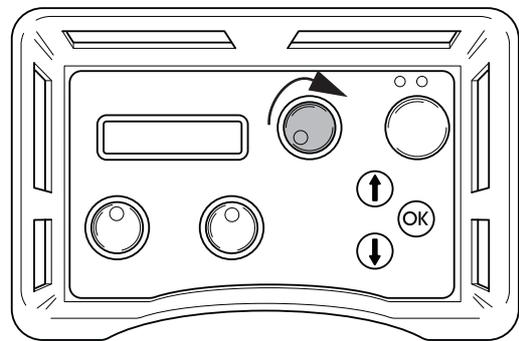
8. Carefully increase the motor speed by turning the control for motor rotation. A suitable working pressure when cutting usually lies between 100 and 130 bar, but varies depending on how many wheel sets are used in the magazine, how much wire is in use and the hardness of the material to be cut.
