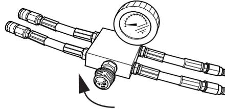
7. Start the motor's rotation by turning the control for motor rotation on the remote control clockwise.
