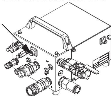
4. Check that the emergency stop on the remote control is not activated. The display on the remote control now shows "SMARTBOX CONNECT HOSE ASSEMBLY"
