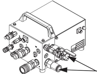
6. If CS2512 is to be used, connect the pressure reduction block's female couplings to the male couplings on RC 455.
