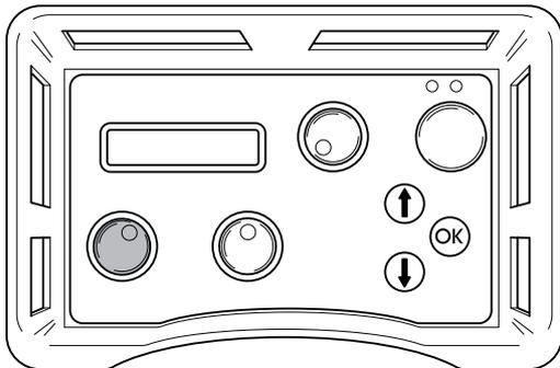
3. Start the horizontal motion by turning the horizontal motion knob in the desired direction.
