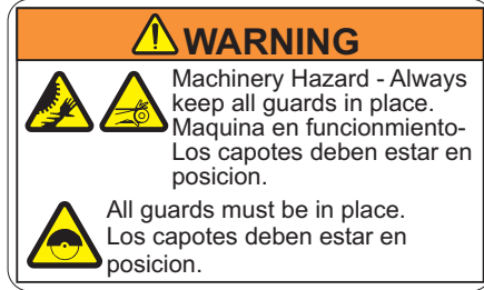
WARNING: 1) Rear of Cowl above opening to transmission, Top of Frame 2) Both Sides of Engine by Lift Bail Mount 3) Front top of Frame, Below Right Angle Gear Box 542 17 62-23* (x4)
