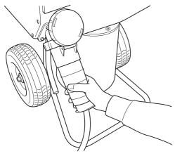
4 Connect the incoming water hose to the water coupling on the bottom of the motor front on the hydraulic unit.
