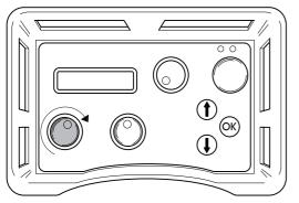
3 Tension the wire by carefully turning the knob on the pressure reduction block clockwise until the wire is tensioned sufficiently. Make sure to always check that the wire is seated correctly in all the wheels on the saw.
