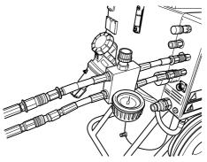
• Close the valve on the pressure reduction block by turning the knob anti-clockwise until it stops and then two turns back.
