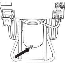
5 Connect the remote control using the supplied Canbus cable. Tighten the cable connector screws by hand.
