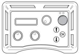
2 Turn the controls for blade rotation and water coolant to their maximum positions to start blade rotation and the water coolant.
