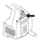
The power switch should be used to start and stop the machine.
