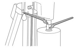
Before the machine is started, carefully check that the new bit is firmly attached.
