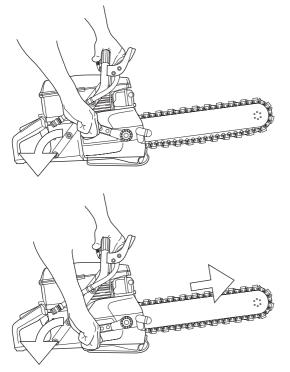
Hold the bar upwards as you move the handle forward.
