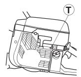
Rec. idle speed: 2700 rpm
