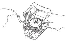
• Secure the starter cord around the cord pulley as illustrated. Tighten the fastening well and ensure that the free end is as short as possible. Secure the end of the starter cord in the starter handle.
