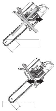
WARNING! Under all circumstances avoid cutting using the side of the chain; it will almost certainly be damaged, break and can cause immense damage. Only use the cutting section.
