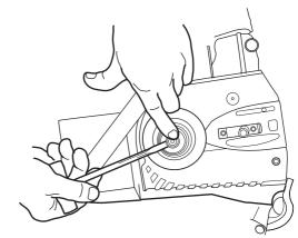
Remove the "halfmoons", the cup guard, o-ring and the drive sprocket.
