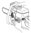
• Fit and tighten the screws that hold the starter.
