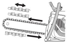
When using a chain with double rakers, the chain can be fitted either way round. When using a chain with one raker, the chain should always be fitted the right way round. The raker should guide the segment at the right height in the cut.
