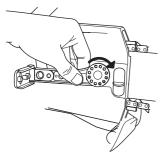
Release the spring. Hold the bar upwards as you move the handle forward. Note that the arm's mechanical stop shall not be reached. The stop prevents the arm from pointing forwards and prevents cutting.
