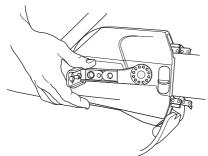
Press the spring down on the chain tensioner handle. Unscrew the adjusting bar nut anti-clockwise.
