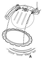
• Press in the guide roller if necessary, so that it climbs into the groove on the blade.
