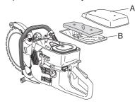
In order to obtain a good filtering effect, the filter must be replaced regularly or cleaned and oiled. A special HUSQVARNA oil has been produced for this purpose.
