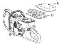
If the machine is low on power, difficult to start or runs poorly at idle speed: always check the spark plug first before taking any further action. If the spark plug is dirty, clean it and check that the electrode gap is 0.020 inch (0.5 mm). The spark plug should be replaced after about a month in operation or earlier if necessary.
