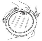
Fit the support roller cover. Now tighten the four screws fully.
