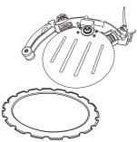
Unscrew the knob. First turn the knob a few turns until you feel a resistance. The guide roller then follows the knob out and stops when it feels a resistance.
