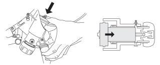
Lubricate the guide roller's sleeve using grease. Fit the grease gun on the grease nipples (A) and pump in grease until clean grease emerges from the overflow hole (B).
