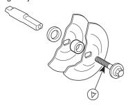
Do not use warped, notched, indented or dirty flange washers. Do not use different dimensions of flange washers.
