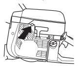
**Stop switch:** Make sure that the stop switch (STOP) is in the left position.
