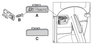
If you want to reactivate the OilGuard system, press the OilGuard plug again. The system is then reactivated, but note that the broken indicator pin cannot be refitted. A broken indicator pin indicates that the OilGuard system has been disconnected. You can purchase a new indicator pin as a spare, but this is only sold in grey which indicates that the OilGuard system has been deactivated since the machine left the factory.
