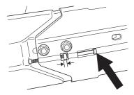
Tighten both of the screws holding the cutting head using a T-wrench.
