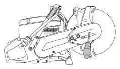
When a diamond blade is mounted on the power cutter make sure that the diamond blade will rotate in the direction indicated by the arrow on the blade.
