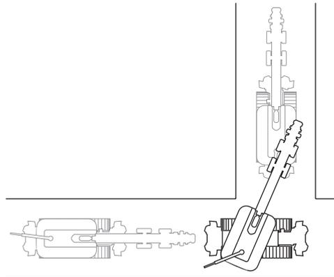
In transport mode, the caterpillar tracks and tower can be maneuvered simultaneously. The function can be used, for example, when the machine is being operated in confined spaces.
