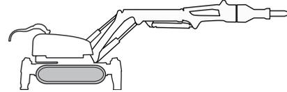
The caterpillar tracks are driven individually by hydraulic motors. The machine can be turned by operating the caterpillar tracks at different speeds. Operating the tracks in different directions enables the machine to make tight maneuvers. When the drive function is not activated the passive brakes lock the drive motors.
