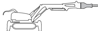
The machine should be fitted with tools that are appropriate for the tasks that are to be carried out. The weight and performance requirement of the tool is decisive in ascertaining whether it is suitable for use with the machine. Further information is available in the 'Tools' and 'Technical data' chapters and the tool supplier's instructions.
