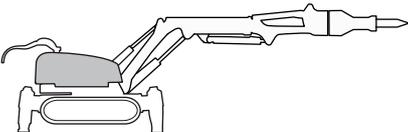
The tower has unlimited rotation, which means that it is possible to work in several directions without having to move the machine. The machine is equipped with a slew brake. When the rotating function is not activated, the function is braked by means of passive brakes.
