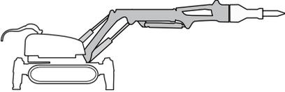
The arm system is divided into three parts in order to provide extensive movement, a long reach and compactness. Expanding shafts minimize the risk of play in the joints.
