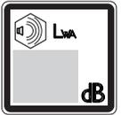
Noise emission to the environment according to the European Community's Directive. The machine's emission is specified in chapter Technical data and on label.
