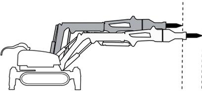
The machine is also equipped with a telescopic arm that provides additional reach. Work as close to the work object as possible as this makes optimum use of the power to the arm system and cylinders.
