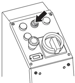
When emergency operation is activated the machine turns off and has to be restarted using the start button on the machine. In this mode the machine can only be moved using emergency operation, other functions are disconnected. When emergency operation is deactivated the machine turns off and has to be restarted using the remote control.
