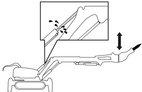
Cylinder 3 is in its outer position and the hammer is working in the downward direction. Never operate the cylinders to their end positions.
