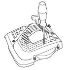
• Lubricate the recoil spring with light oil. Fit the pulley and tension the recoil spring.
