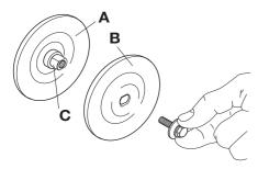
The shaft can be locked using a screwdriver, steel pin or the like. This is slid in as far as possible. The blade is tightened clockwise.
