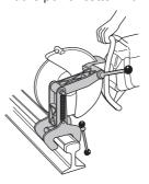
Guide the cutting blade down towards the rail and check that the cutting blade is centred in the cut. If necessary, adjust the movable bushing so that the blade ends up centred in the middle of the cut.
