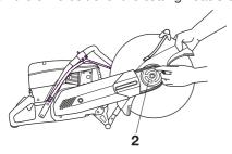
Screw the rear belt cover in place and lock into place the cutting head together with the front belt cover.
