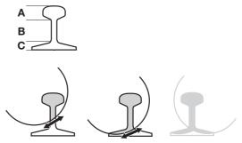
If the cut cannot be completed from one side, the power cutter must be turned around.
