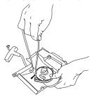
• Undo the screw in the centre of the pulley and remove the pulley. Insert and fasten a new starter cord to the pulley. Wind approx. 3 turns of the starter cord onto the pulley. Connect the pulley to the recoil spring so that the end of the spring engages in the pulley. Fit the screw in the center of the pulley. Insert the starter cord through the hole in the starter housing and the starter handle. Make a secure knot in the end of the starter cord.
