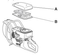
Remove the foam plastic filter. Wash the filter well in tepid soapy water. After cleaning, rinse the filter well in clean water. Squeeze out and allow the filter to dry. NOTE! High pressure compressed air can damage the foam.
