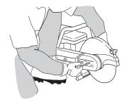
Tightening torque for the bolt holding the blade is: 15-25 Nm (130-215 in.lb).
