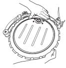
• Fit the support roller cover. Now tighten the four screws fully.
