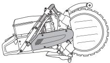
• Press on the belt tensioner with your thumb to tension the belt. Now tighten the screw holding the belt tensioner.
