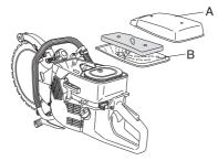
If the machine is low on power, difficult to start or runs poorly at idle speed: always check the spark plug first before taking any further action. If the spark plug is dirty, clean it and check that the electrode gap is 0.5 mm. The spark plug should be replaced after about a month in operation or earlier if necessary.
