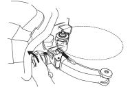
The guide roller can now be pulled out of the chassis
