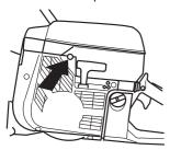
**Stop switch:** Make sure that the stop switch (STOP) is in the left position.
