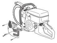
Undo the bolt in the centre of the pulley and remove the pulley.
