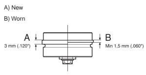
• Replace the support rollers when the roller surface is flat, (or) when the groove on the roller surface has worn away.
