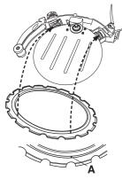
• Press in the guide roller if necessary, so that it climbs into the groove on the blade.
