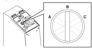
To activate the remote control mode, turn the knob to the left (A).
