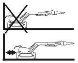
Do not work with the machine's cylinders in the inner or outer end positions to avoid overloading. Leave a few centimeters to the maximum position. The hydraulic fluid then has a greater capacity to alleviate impacts and vibrations. • There are two working positions that put a lot of strain on individual cylinders.
