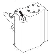
Place a collecting vessel under the tank's drain plug and open the plug.
