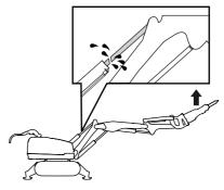
Cylinder 3 is in its outer position and the hammer is working in the downward direction. Never operate the cylinders to their end positions.
