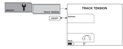
Hold the selection key down to activate the track tension.
