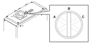
To activate the remote control mode, turn the knob to the left (A).
