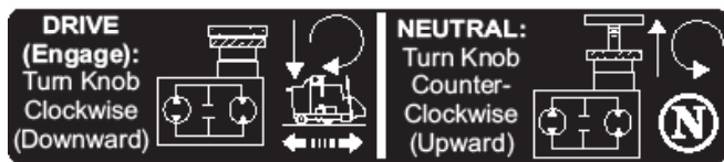
TRANSMISSION BYPASS VALVE FRAME - NEAR VALVE 542 19 06-28
