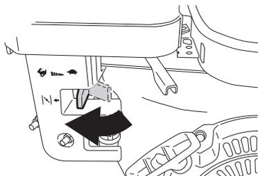
The closed choke position enriches the fuel mixture for starting a cold engine.
