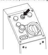
When emergency operation is activated the machine turns off and has to be restarted using the start button on the machine. In this mode the machine can only be moved using emergency operation, other functions are disconnected. When emergency operation is deactivated the machine turns off and has to be restarted using the remote control.
