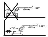
Do not work with the machine's cylinders in the inner or outer end positions to avoid overloading. Leave a few centimeters to the maximum position. The hydraulic fluid then has a greater capacity to alleviate impacts and vibrations.  There are two working positions that put a lot of strain on individual cylinders.
