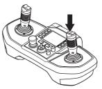
If no command is given within three seconds the operating functions are locked. To return to work mode, press the left button on the right joystick.
