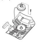
Bear in mind that the return spring lies tensioned in the starter housing. · Loosen the bolts holding the spring cassette.
