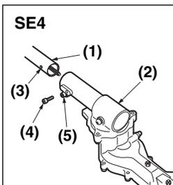
1. Remove the screw screwed into the end of the trimming mechanism.
