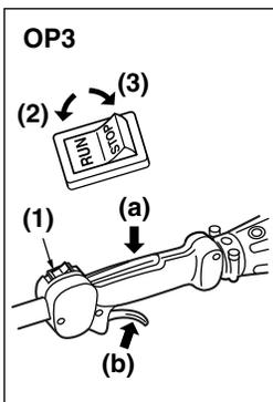
4. Set the stop switch to the "RUN" position. Place the unit on a flat, firm place. Keep the cutting head clear of everything around it. (OP3)
