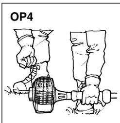
5. Firmly grasp (a) and (b) with left hand (OP3), pull the starter knob quickly until engine fires. Release throttle trigger after engine starts. (OP4)
