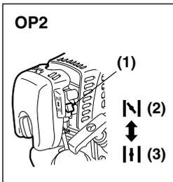
3. Move the choke lever to the closed position. (OP2)
