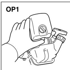
2. Push the primer pump several times until overflow fuel flows out in the clear tube. (OP1)
