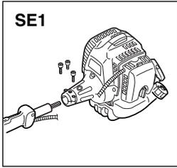
1. Push the driveshaft housing toward the clutch housing and rotate it by hand to check that the driveshaft is engaged with the gears.
