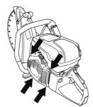
Pull the cord out about 30 cm and lift it into the cut-out in the periphery of the starter pulley. When the cord is intact: Release the spring tension by letting the pulley rotate slowly backwards.
