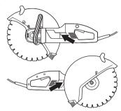
Unscrew the cable holding the carbon brush. Now lift up the spring and then lift out the carbon brush from the brush retainer.
