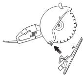
Make sure the locking catch rests upon the lug on the cover. Flip up the locking catch and press it against the protective cover.
