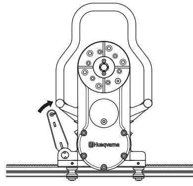
**WARNING!** To cut without the saw securely assembled in the saw carriage and rail is associated with mortal danger.
