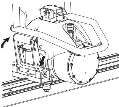
Then secure the locked handle with the locking pin.
