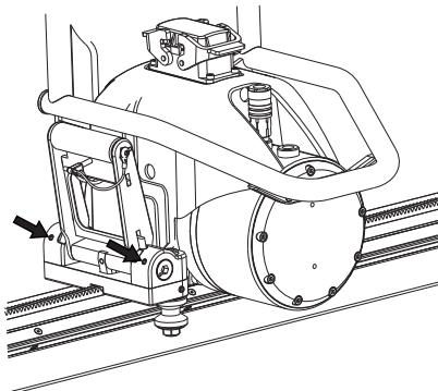
Make sure the locking handle is properly adjusted by open and close and see that the spring loaded lock is in locked position.
