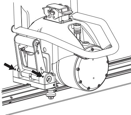
Turn the two excenter sleeves with a 8 mm allen key until the shaft is tight and parallel to the saw unit.
