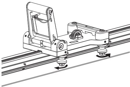
Hold the 16 mm wrench in position and tighten the two stop screws with a 3 mm allen key.
