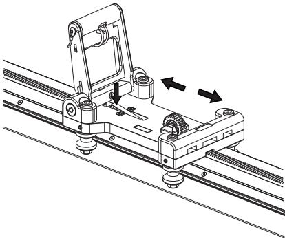
Tighten screws with a 8 mm allen key. Repeat the previous step.
