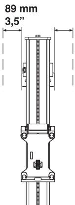
**IMPORTANT!** Only use the connectors supplied when purchasing the saw as older connectors are not designed for the WS 400 series.
