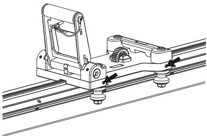
Press down the locking device and pull the saw carriage in both directions by hand. Carriage should slide easily with a slight resistance. All 4 guide wheel should spin.
