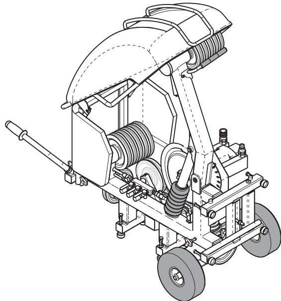
Husqvarna CS 2512 is designed for use together with the hydraulic unit PP 455 E or Husqvarna RC 455. Husqvarna CS 2512 is a powerful and easy to use wire saw with a capacity for really large work, yet at the same time sufficiently compact and mobile for small work. It can be used in many different ways, both on the ground and fitted to the wall.
