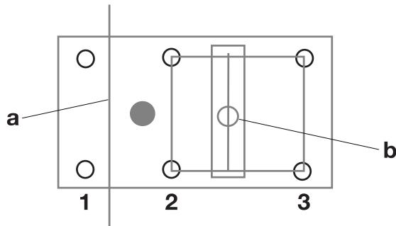
If necessary, fit pulley wheels to assist the cutting process. Using the pulley wheels allows the number of sharp corners that the wire must be pulled around can be reduced, which results in less wear to the wire at the same time as cutting is made easier. Using the pulley wheels also lets the wire be guided in different directions without the need of moving the saw unit.
