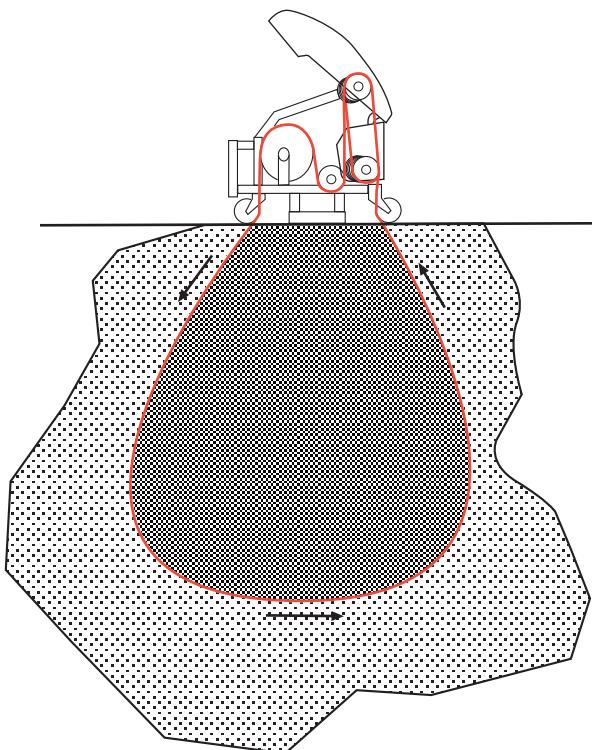
It may be necessary to drill holes to thread the wire through the material to be cut.
