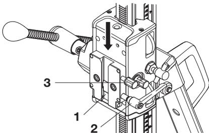
Use top positioned locking screw (3) only together with DMS 240.
