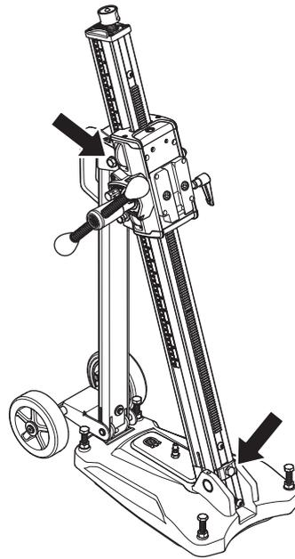
Loosen the locking screws for column tilt and set the desired drill angle. Tighten the locking screws. Use the feed handle. The column can be tilted 0-60°.
