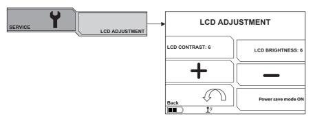
Use the arrows up and down to adjust the display's contrast and brightness.
