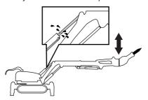
Cylinder 3 is in its outer position and the hammer is working in the downward direction. Never operate the cylinders to their end positions.
